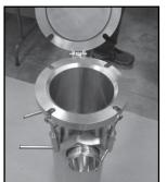
Custom Hi-Capacity Basket Strainer -3.8 s/f basket area with bevel seat connections and a swing bolt top cover; pressure tested to 300 psi.
