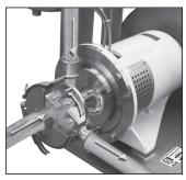
The in-line SLIM system replaces older technology that relies on an eductor to draw powders into a liquid stream. The result – much faster induction rates and virtually no clogging!
