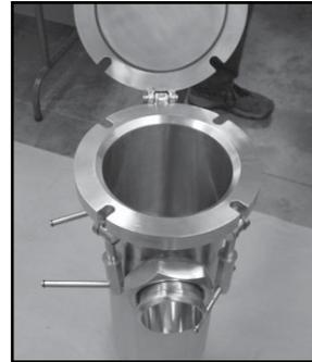
*Custom Hi-Capacity Basket Strainer - 3.8 s/f basket area with bevel seat connections and a swing bolt top cover; pressure tested to 300 psi.*
