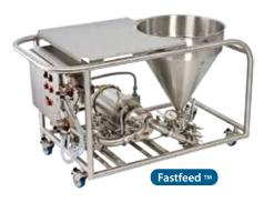
Our ergonomic **Fastfeed™ powder induction system** offers rapid atmospheric powder conveying, feeding, and dispersion in a fully-automated, integrated package. This skid-mounted system uses a specially designed suction pump and delivers controlled feed rates up to 450 pounds per minute. Visit **admix.com/fastfeed** for more info.
