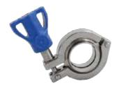
Trynox Clampsense™ is intented to mitigate the possibility of cracking or gasket debris. Fits to sanitary stainless steel tubing, surface finishing 150 Grit OD. Has a maximum operating pressure rating of 140 psi at 70 degrees F ambient tempeture.
