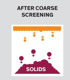
Larger particles in a DAF are harder to float and, despite chemical assistance, they can sink to the bottom requiring costly, manual cleanouts. SOLIDS TEQUATIC<sup>™</sup> PLUS Filters increase DAF efficiency and float consistency by delivering particles to the DAF that are in a more optimal size range
