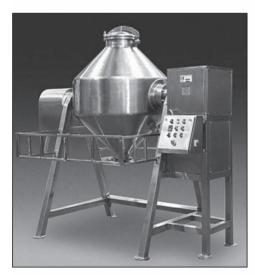
Blending cycles are fast – typically 10 minutes or less – with Ross Double Cone Blenders. Standard sizes from ½ to 80 cu.ft. are available, and many are in stock for immediate delivery. Type 316 stainless with 240-grit interior polish.
