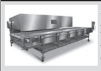
Extremely uniform treatment with shorter melt/ fuse times eliminating ingredient damage. Runs on infrared alone thus minimizing any disturbance of ingredients as they pass through. Stainless steel wire belt conveyor is removable for ease of cleaning. Wash-down design. Available in various widths and lengths to suit production requirements. Quick payback on investment.
