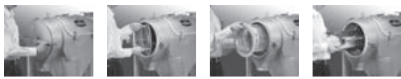
Opening a hinged door at the discharge end of the screening chamber allows a retainer plate, screen cylinder, and helical paddle/feed screw assembly to be removed quickly and easily.
