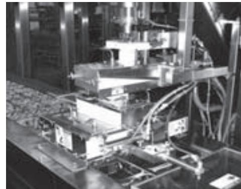
The MPF distribution system has been designed to distribute small dimensioned, hard to fill products such as cooked rice and pastas, vegetables, fruits and salads into various patterns.
