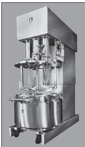
*Ross can also provide a High Shear Mixer incorporated in an advanced sanitary multi-agitator mixer. With supplemental agitation, the High Shear Mixer's operating range easily extends to 200,000 centipoise – at least ten times higher than a rotor/stator mixer operating alone.*
