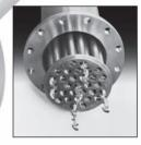
In the ISG Static Mixer, four holes bored through the elements provide flow paths that separate and recombine viscous material and achieve complete homogeneity.
