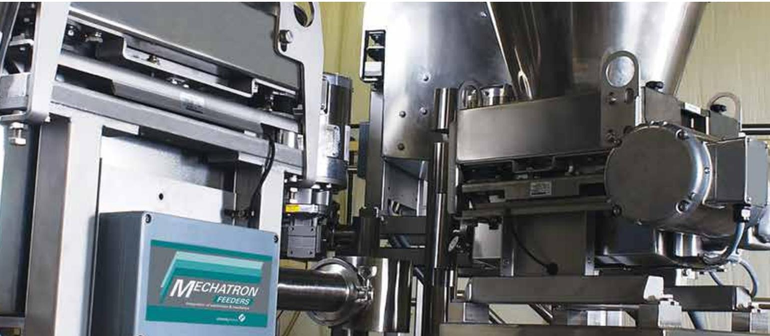
The uniquely designed MECHATRON® is the only feeder on the market that can be completely disassembled from the non-process side of the feeder in a matter of minutes. This eliminates the need to remove upper extension hoppers, bins, bulk bags, and IBC's to clean or maintain the feeder, saving time and money! Plus, the MECHATRON® can be equipped with best-in-class controllers and extended helixes and nozzles for challenging feeding applications. Contact us for more information.
